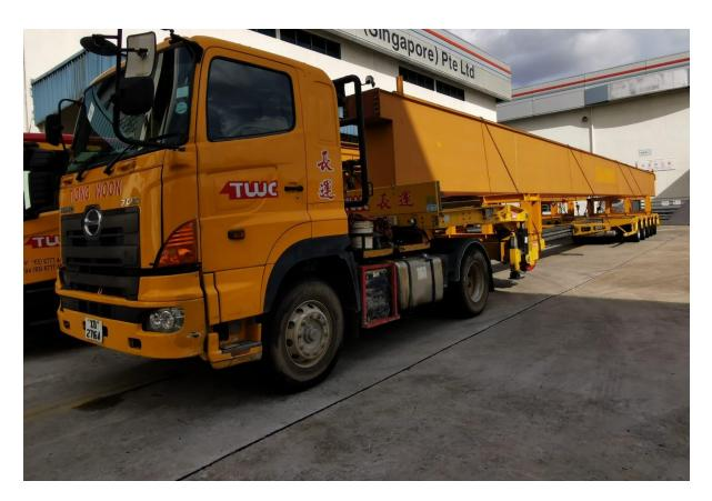
Our client initially chose to load all three Girders on one Self-Propelled Modular Transporter (SPMT) for this project. However, after accessing the risks, dimensions, and nature of the load, we suggested using the extendable loaders for the three Girders' transportation. The team advised distributing two Girders to one loader, and the other carrying one.
