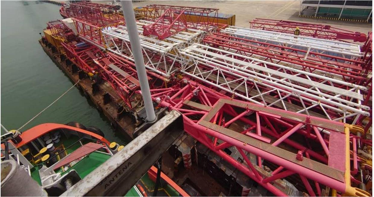
With a total laden weight of 3,300Tons of assets on the Barge, Tiong Woon Ocean 18, a Brake Horsepower (BHP) of 3200BHP was chosen to tug Tiong Woon 32, a barge that has a maximum Deadweight Tonnage of 5,500Tons, back to Singapore.
