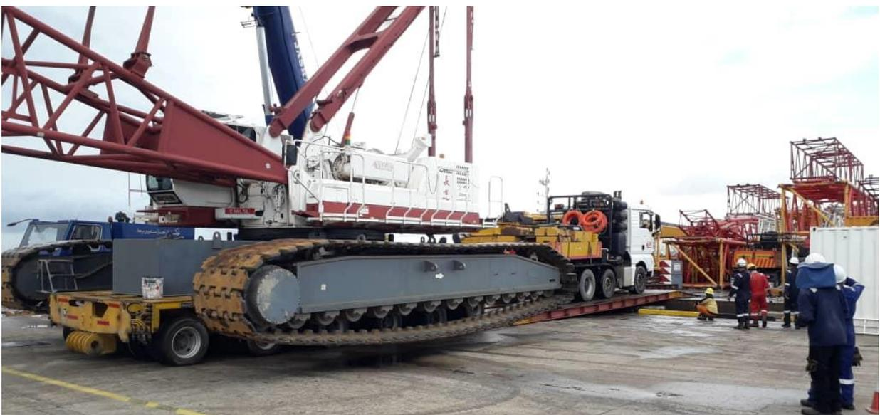
Once all assets are onboard, the Mobile crane decoupled the rams from the barge and the marine team finalized the lashings for the RORO operation to commence.
