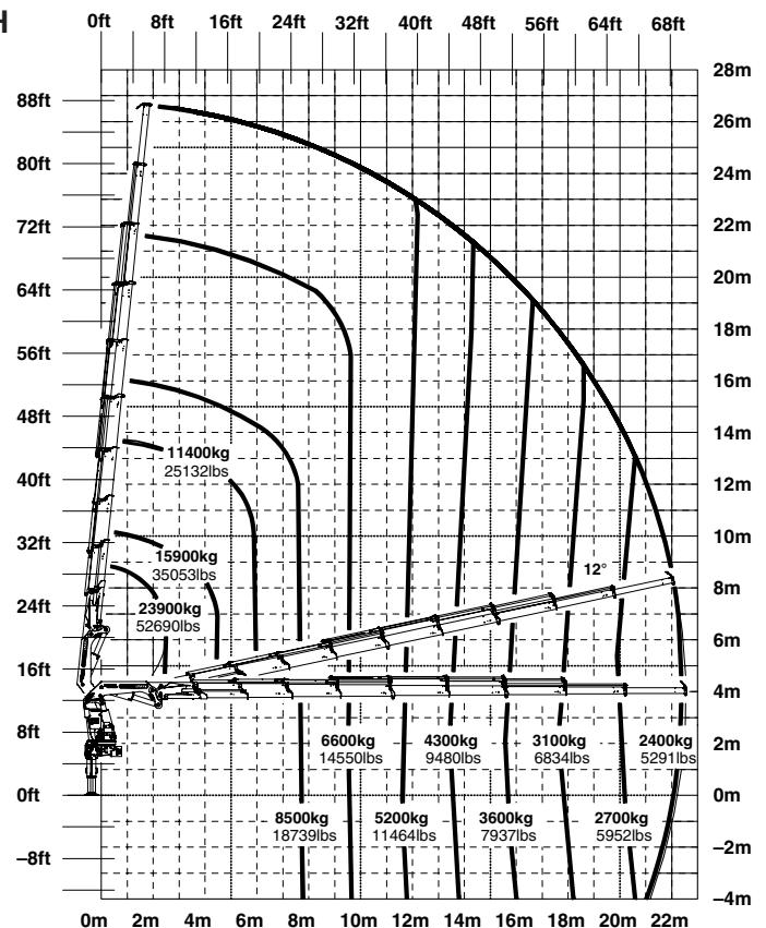
The outreach values stated are with a boom angle of 20° and are therefore not the maximum.
