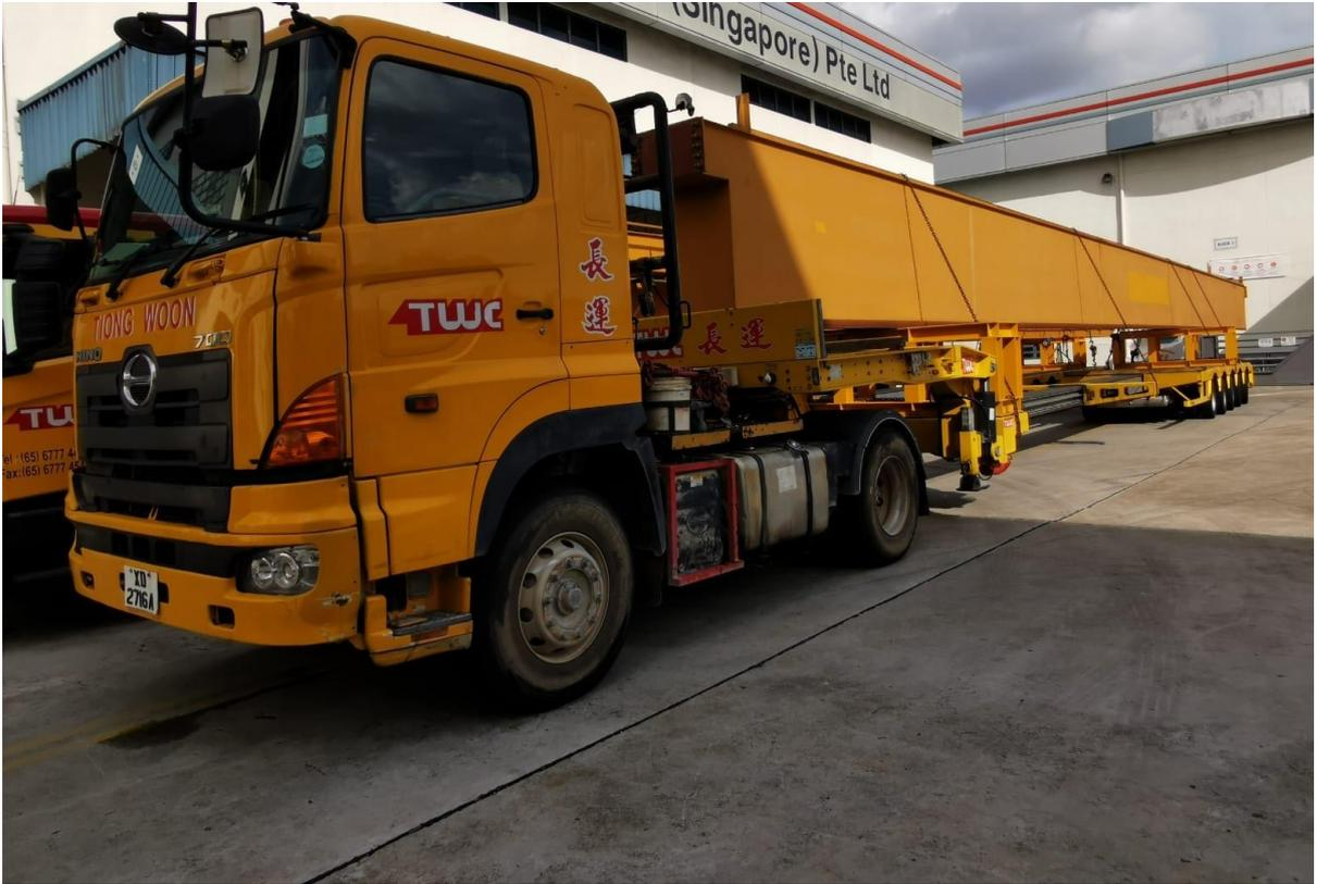
Our client initially chose to load all three Girders on one Self-Propelled Modular Transporter (SPMT) for this project. However, after accessing the risks, dimensions, and nature of the load, we suggested using the extendable loaders for the three Girders' transportation. The team advised distributing two Girders to one loader, and the other carrying one.
