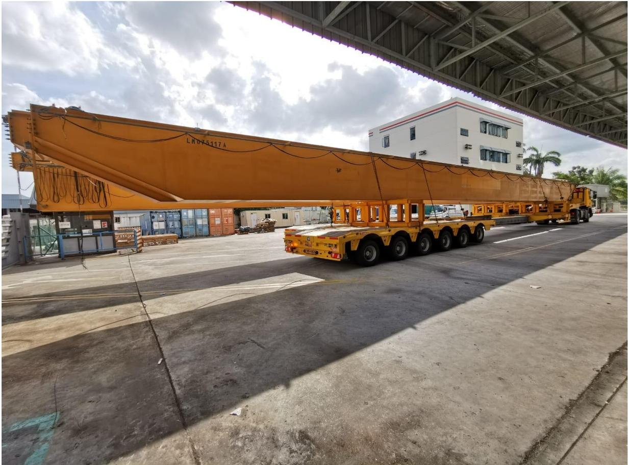
The transport team had to plan the vehicle's precise movements, ensuring the turning radius is big enough for the loaders to turn out from the loading site and turning into the unloading site.
