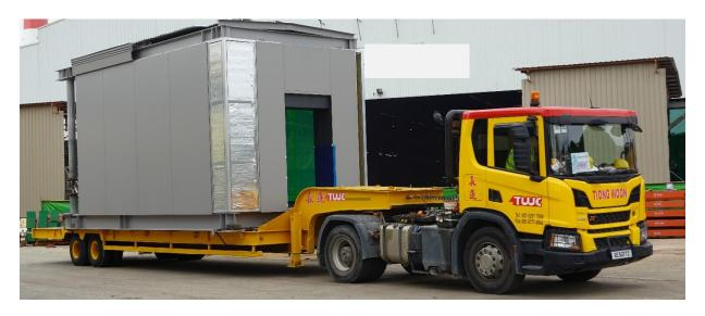
Measuring 21.42m (L) x 3.28m (W) x 4.3m (H) & weighing 52.6 Tons for the longer frame, 7.76m (L) x 3.7m (W) x 4.2m (H) & weighing 19.4 Tons for the shorter frame, we deployed a 12-axle Cometto connected to a Prime Mover to transport the longer frame. A Prime Mover with a Low Bed Trailer was deployed to transport the short frame.
