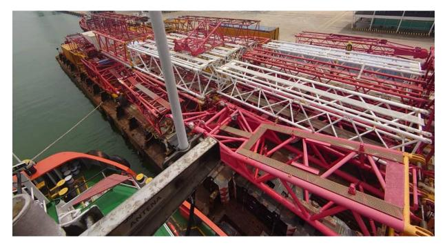
With a total laden weight of 3,300Tons of assets on the Barge, Tiong Woon Ocean 18, a Brake Horsepower (BHP) of 3200BHP was chosen to tug Tiong Woon 32, a barge that has a maximum Deadweight Tonnage of 5,500Tons, back to Singapore.
