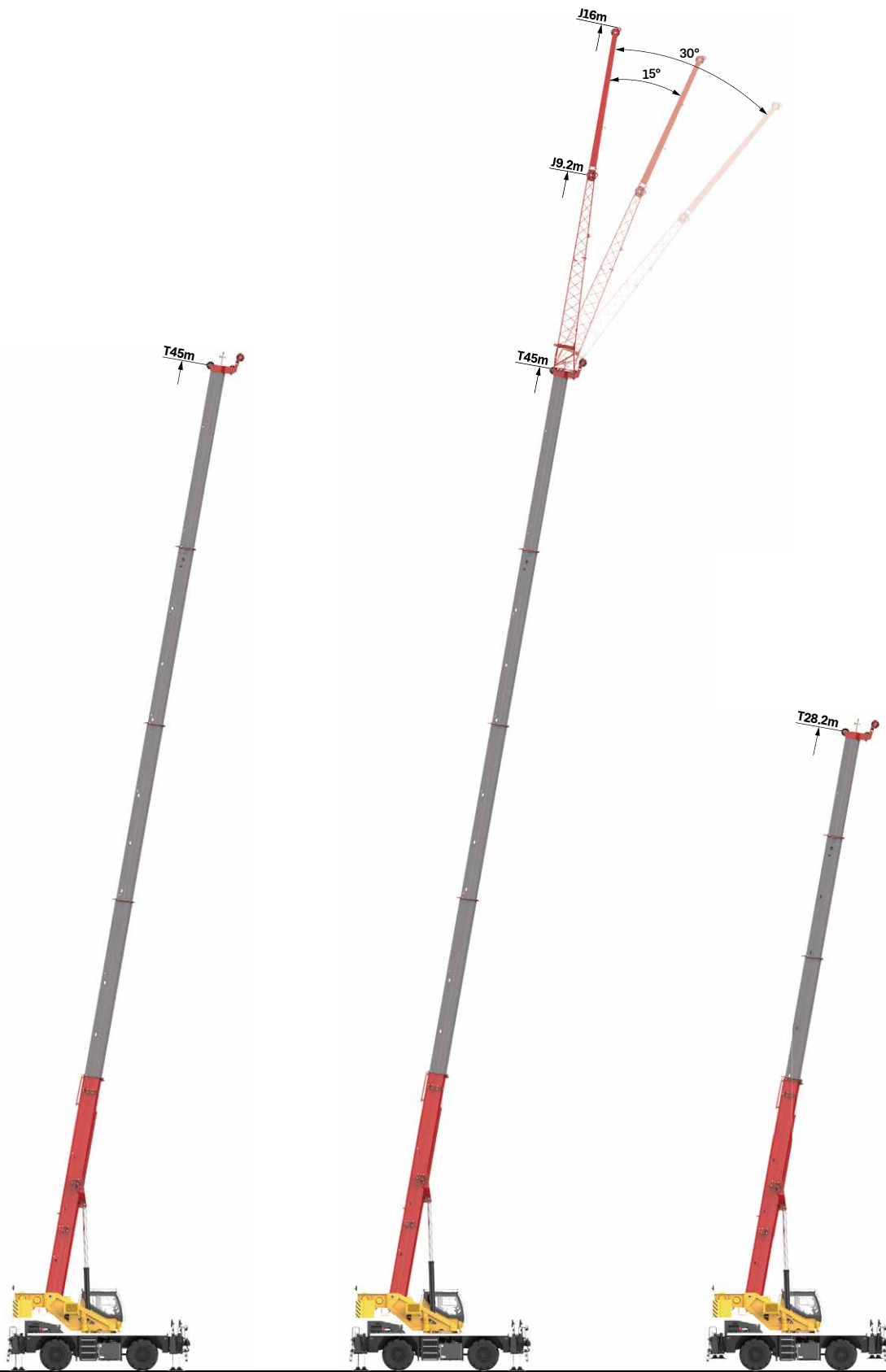
Telescopic boom on outriggers 主臂、支腿吊载
