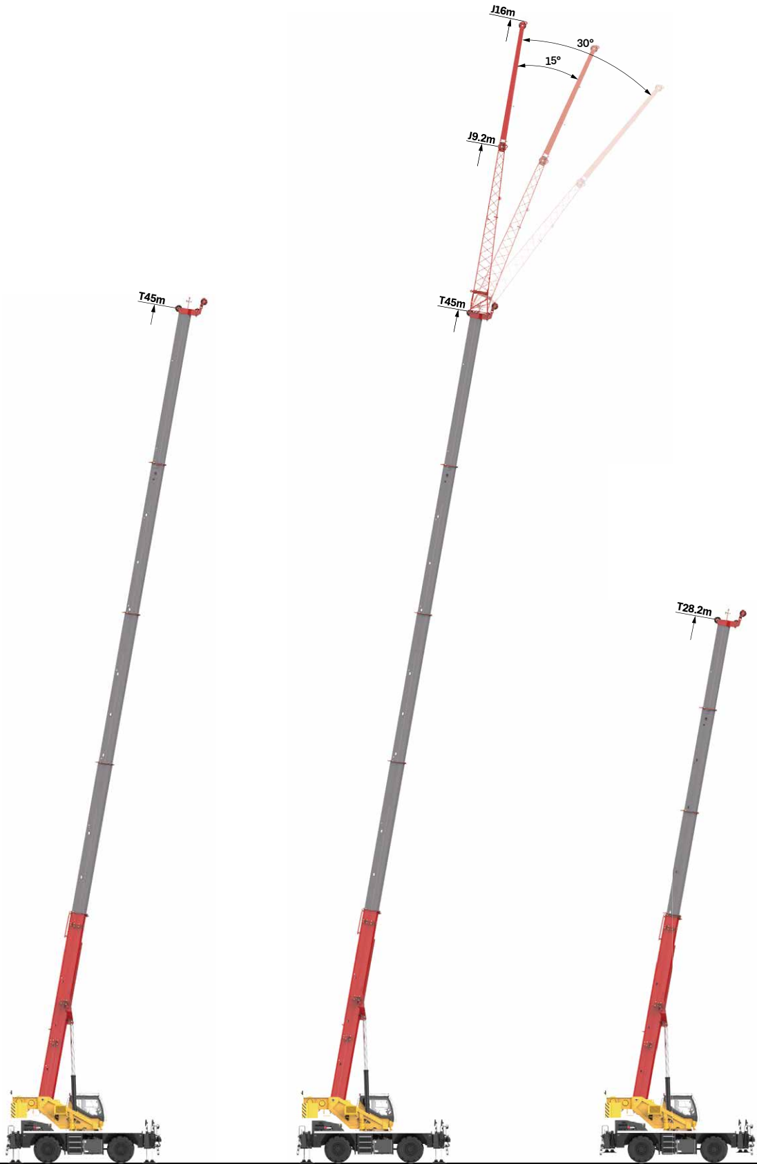
Telescopic boom on outriggers 主臂、支腿吊载
